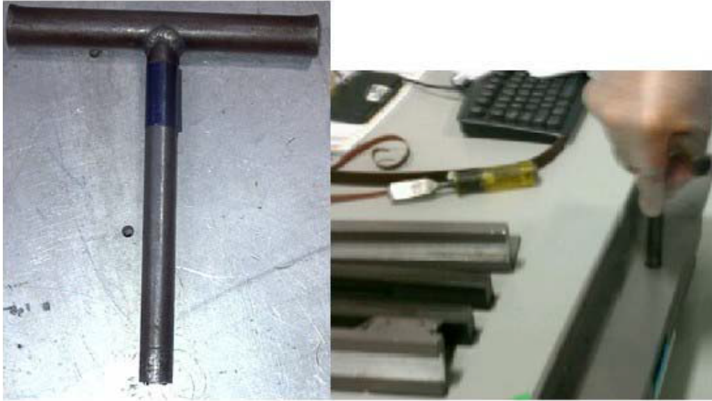
T-Bracket Shop Aid Tool Figure 6002/GRAPHIC 25-20-45-300-002-A01
